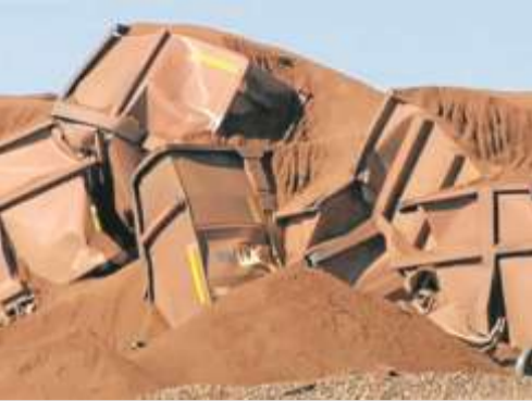
The cause was a combination of brake system failure and incorrect operating procedure. Picture: Seven News
