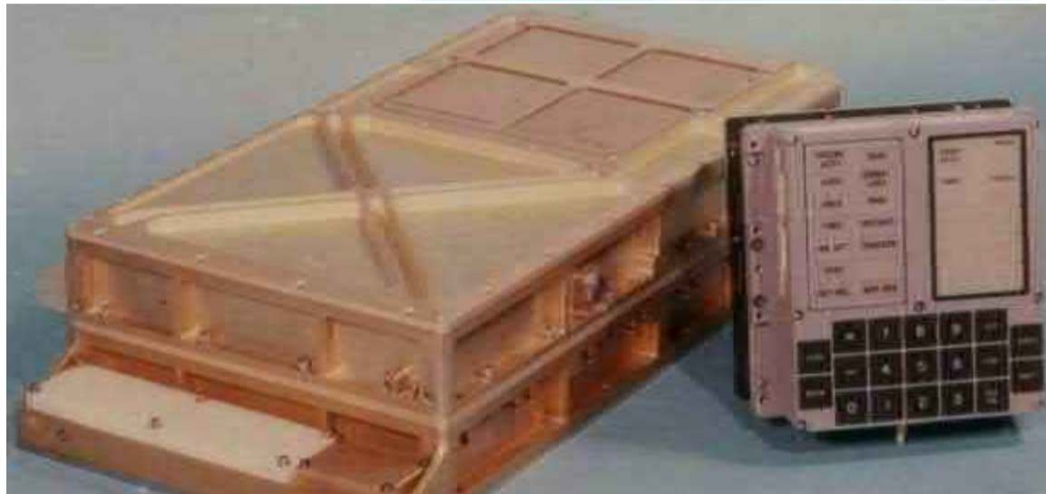
The DSKEY input module (right) shown alongside the Apollo Guidance Computer's main casing (left). Apollo 11 computer 100,000 times less powerful than iPhone used to mine Bitcoin
