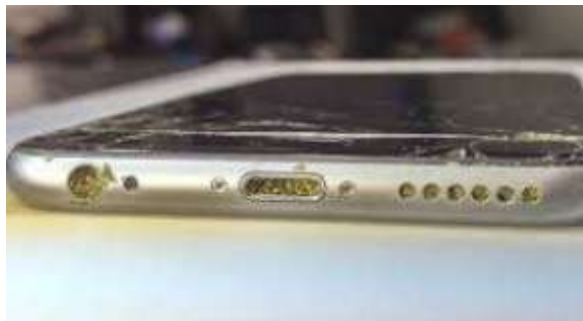
Rice stuck in the vents and holes.
