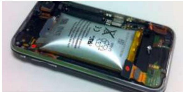
This battery is swollen. It can lead to the screen popping off, lifting and cracking. It can also lead to the phone exploding and igniting.
